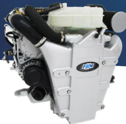
FNM® 4-cylinder 20HPE marine engine is based on the new 2LT Multijet engine, that equips a large number of small and medium size cars in Europe. The engine uses a common-rail fuel injection system controlled by an ECU (Electronic Control Unit), especially made for it. The engine is small and powerful, its wide distribution is the proof of its reliability and wide availability of spare parts.
